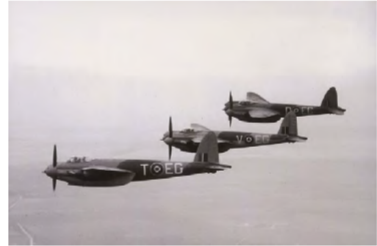
Mosquitoes from Pickard's squadron. Primarily built from plywood, canvas and glue. At 380 mph, one of the fastest bombers/fighters of WW11.
